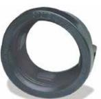
**Open Grommet** 91400 Fits 2 1/2" round lamps Fits panel thickness up to 1/8"
