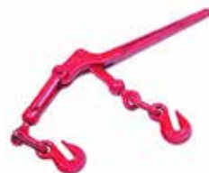
5/16-in. Lever Load Binder Weight: 7.9 lbs./3.59 kg WLL: 5,400 lbs./2,450 kg 45943-10
